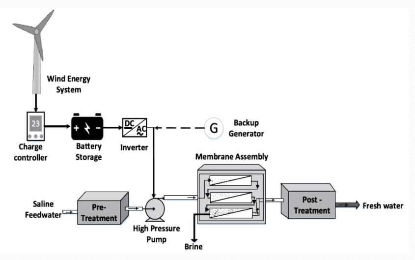
Schematic representation of a typical wind-RO desalination system 16
