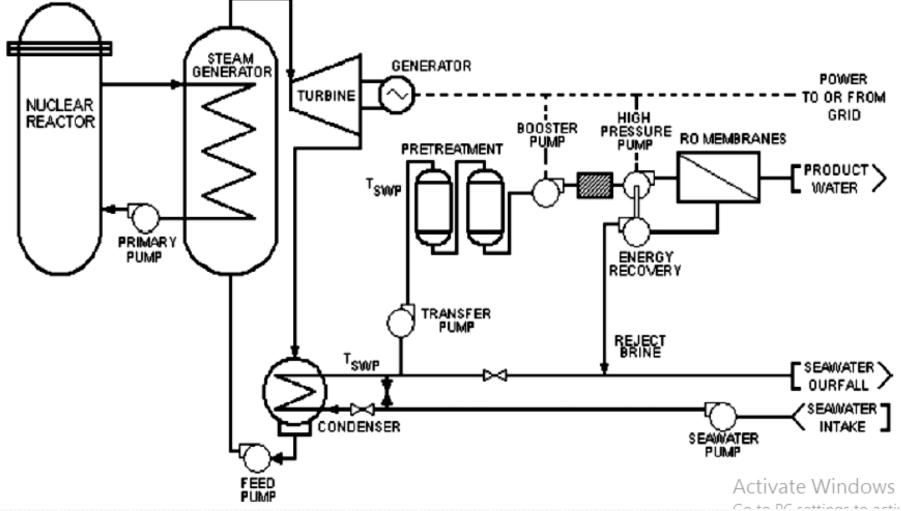
Schematic representation of nuclear power plant powered RO desalination plant
