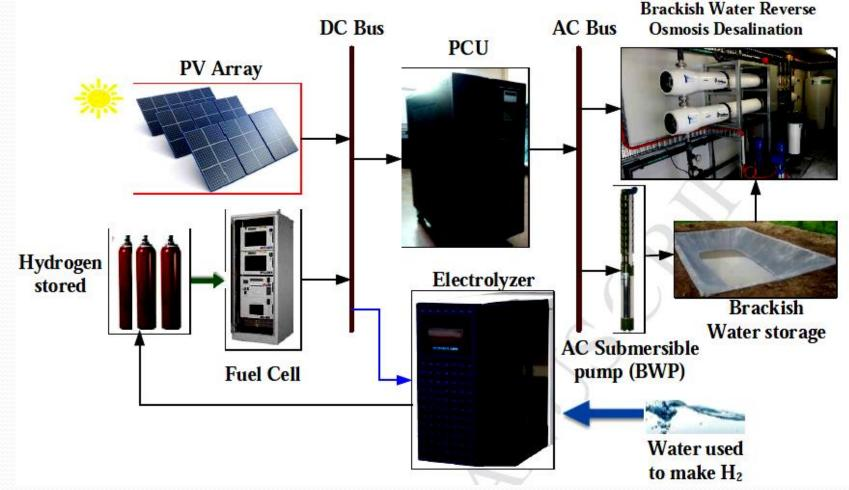
The system consists of PV array, self-charging fuel cell, electrolyzer, power conditioning unit (PCU) and hydrogen storage tank. 3
