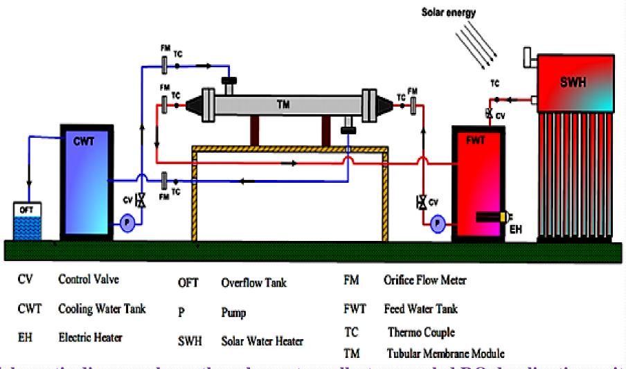
Schematic diagram shows the solar water collector coupled RO desalination unit
