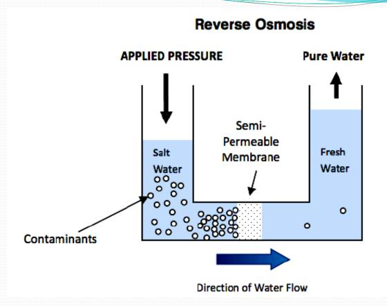
When pressure is applied to the concentrated solution, the water molecules are forced through the semi-permeable membrane from concentrated solution to fresh water. The amount of pressure required depends on the salt concentration of the feed water. The more concentrated the feed water, the more pressure is required to overcome the osmotic pressure.
