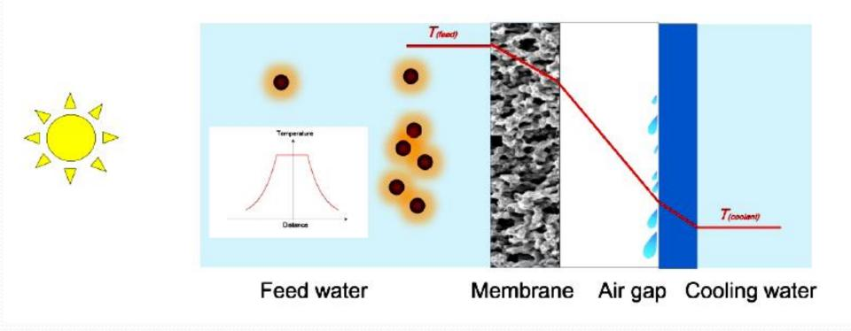
The nanofluid enhanced solar-powered membrane distillation represents a promising perspective for better solar energy utilization.
