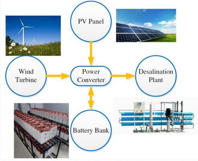
Schematic of a typical small hybrid solar-wind-powered desalination plant. 18
