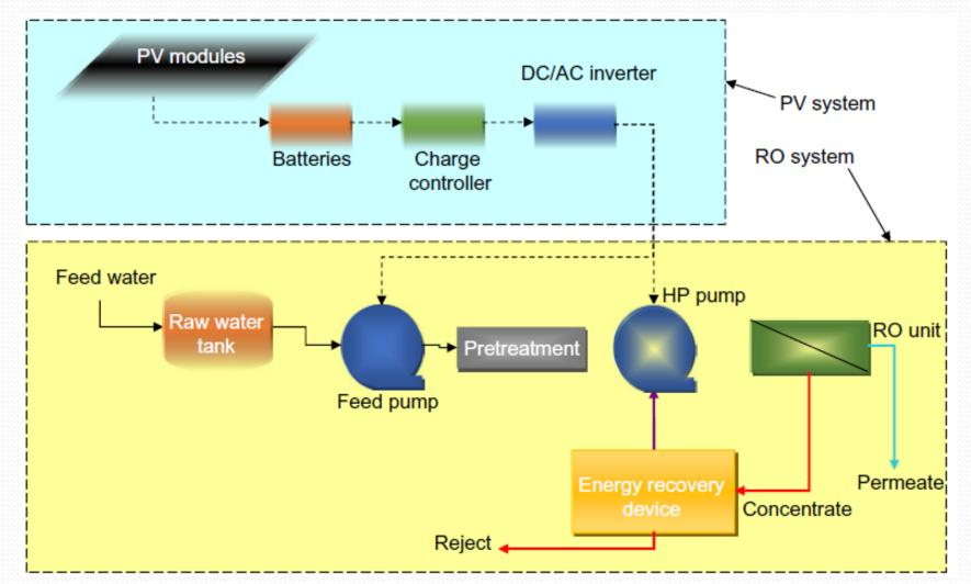
Basic design model of a RO water desalination system powered by PV.
