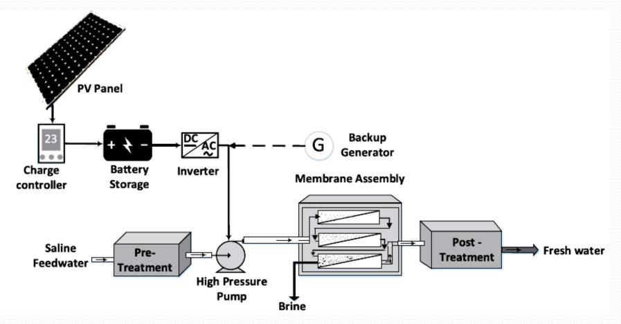
A schematic representation of a PV-RO system
